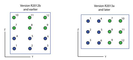
New Size and Element Indexing Order for Replicated URA [3,2] Subarrays Example: GridSize = [1,2]
